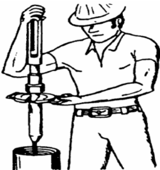
Figure 11 (The C-plate is placed in the slot between rope socket and spear.)
