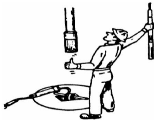
Figure 7 (Pick up the cable to monkey board by wire line hoist)
