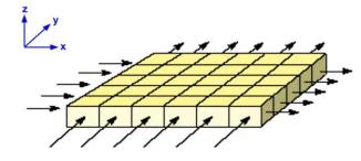
$$1.127 \times 10^{-3} \left[ \frac{\partial}{\partial x} \left( \frac{k_x}{\mu} \frac{\partial p}{\partial x} \right) + \frac{\partial}{\partial y} \left( \frac{k_y}{\mu} \frac{\partial p}{\partial y} \right) \right] - \frac{q_{sc}(x, y, t)B}{V_b} = \frac{\phi c_t}{5.615} \frac{\partial p}{\partial t},$$
