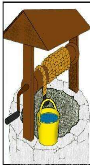
A Windlass hoists water from a well
