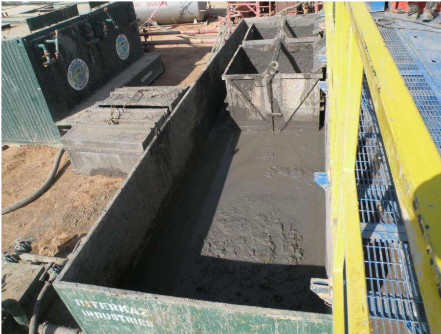
Figure: (3-9) WASTE PIT
