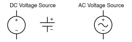
Electrical energy is distributed through the power grid as alternating current, but electronic systems require DC supply voltages. An AC supply voltage can be converted into a stable DC supply voltage by means of a rectifier followed by a voltage regulator. We'll learn more about AC-to-DC conversion and voltage regulation in future video tutorials.
