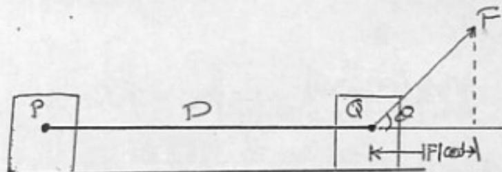
$$\text{Work} = (\text{scalar component of } F \text{ in the direction of } D) (\text{length of } D)$$
