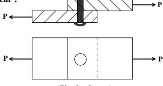
*d* ------ Diameter of area parallel to load direction (m) .
