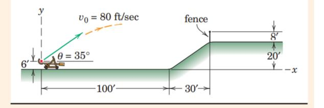
**Solution**. We make the assumptions of constant gravitational acceleration and no aerodynamic drag. With the latter assumption, the 8-lb weight of the projectile is irrelevant. Using the given x-y coordinate system, we begin by checking the y-displacement at the horizontal position of the fence.
