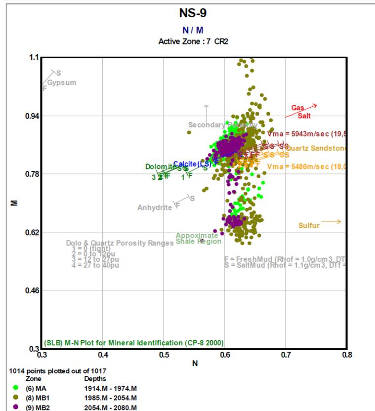
Figure 10: The M-N Cross Plot for Mineral Identifications for (well-9).
