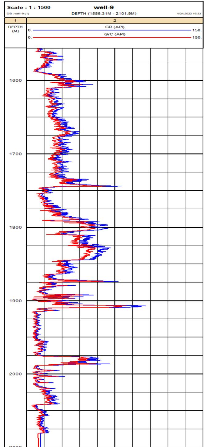
Figure 8. Gamma ray log correction for (Well-9)
