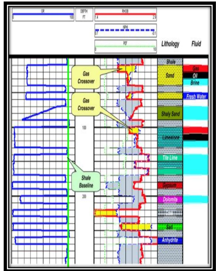
Fig.6: Schematic nuclear-log responses for some common lithologies.
