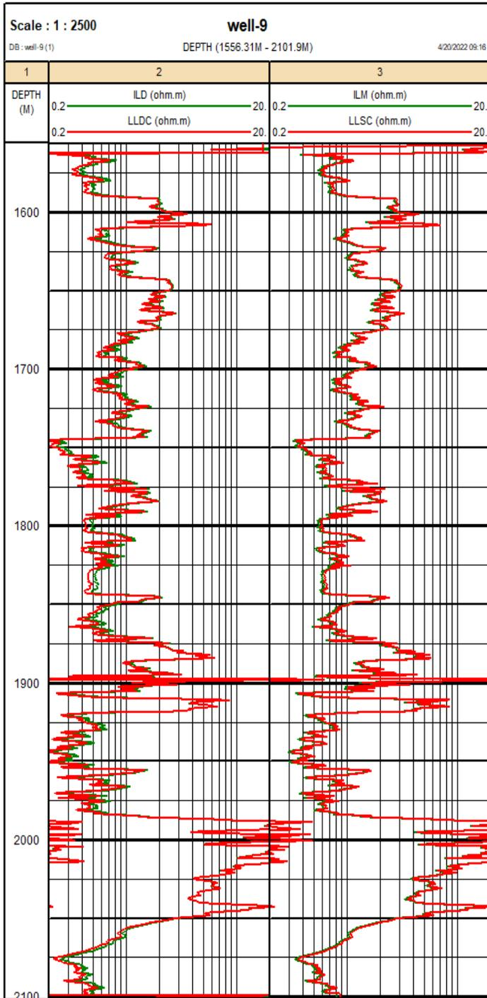
Figure7. Resistivity log corrections for (Well-9)
