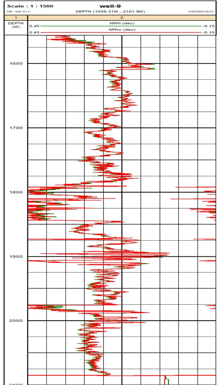
Figure 11: Neutron and density logs corrections
