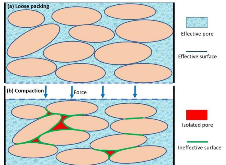
Figure 3: Illustration of the effective porosity and effective specific surface area when the compressible bed is under compaction (b) in contrast to the bed at loose packing condition (a).
