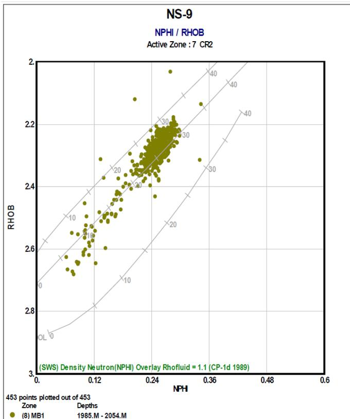
Figure 9: Neutron-density crossplot showing where the common lithologies for (well-9).
