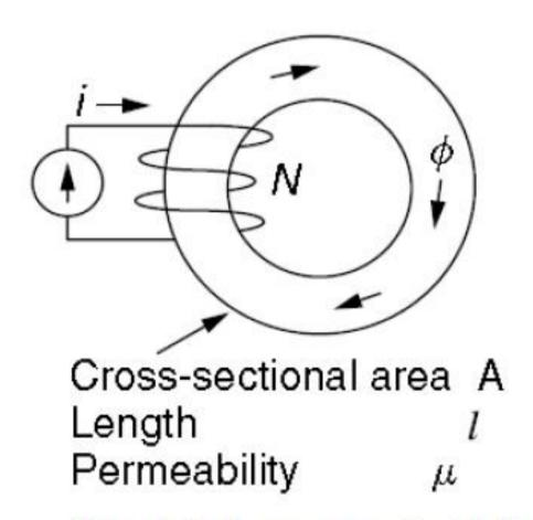
Figure 1 Analogous magnetic circuits.
