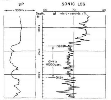
5. Estimate the average porosity of the thick sand interval shown on the sonic log of figure below. (20 pts).
